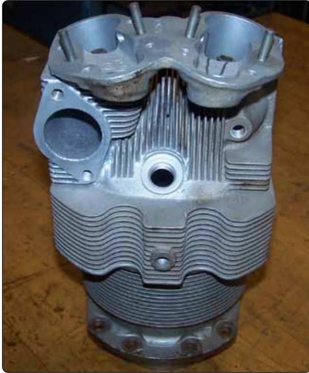
Figure 1-16. An example of an engine cylinder.
