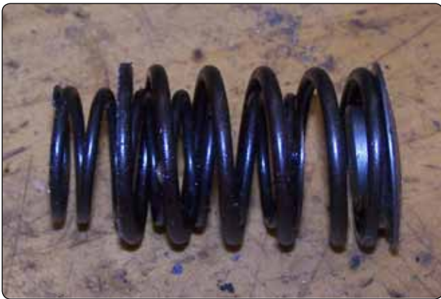
Figure 1-26. A typical set of valve springs used to dampen oscillations. Multiple springs are used to protect against breakage.
