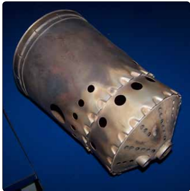
Figure 1-52. Can-type combustion chamber.
