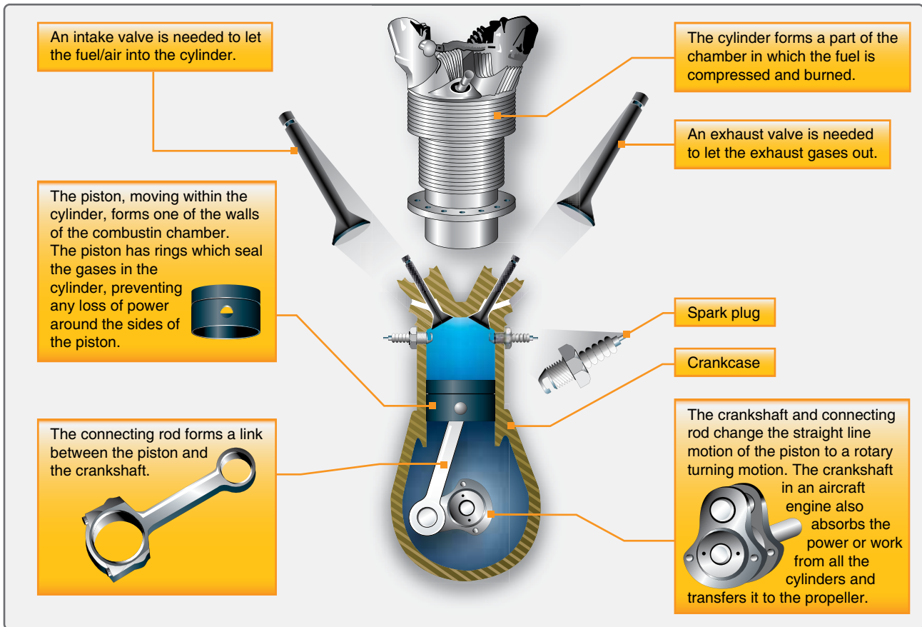
Figure 1-4. Basic parts of a reciprocating engine.
