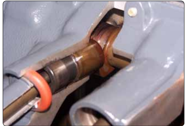
Figure 1-29. Cam load on lifter body.
