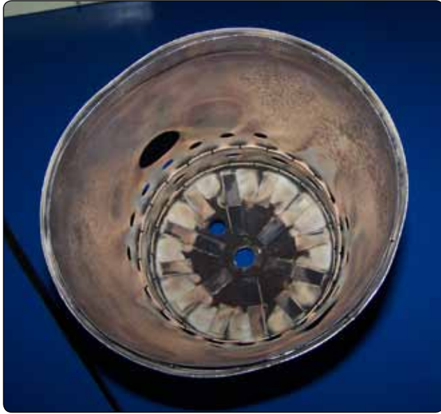
Figure 1-53. Inside view of a combustion chamber liner.
