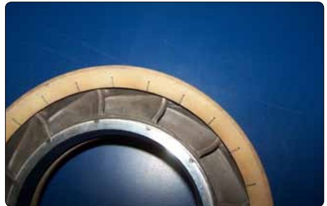
Figure 1-60. Turbine inlet guide vanes.
