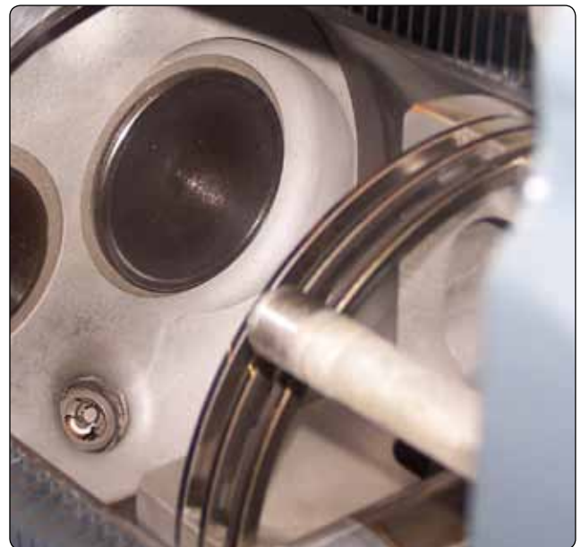
Figure 1-15. Machined rings around a piston.
