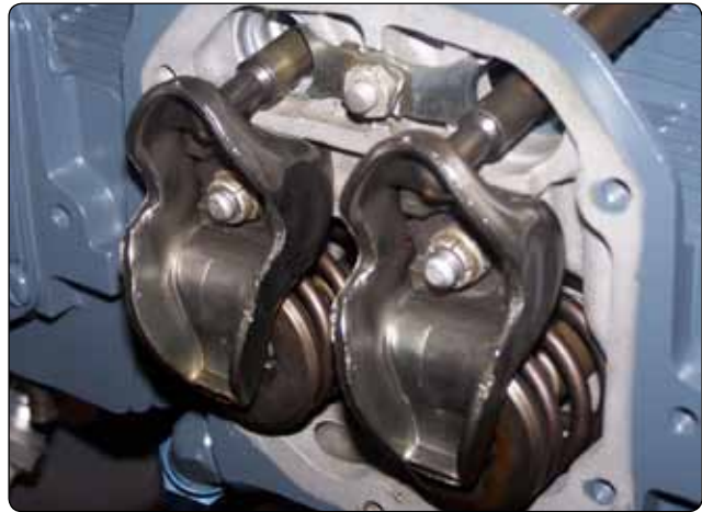
Figure 1-31. Rocker opposed engine arms.
