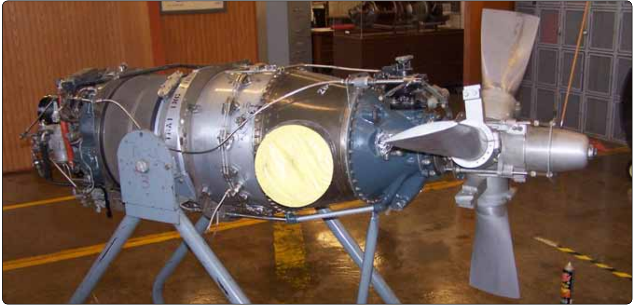
Figure 1-77. PT6 turboprop engine.
